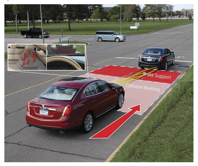
This is a technique for applying technology and automation to prevent human error. In the example above, the target vehicle is set up with sensors to detect the distance to the previous car to reduce the likelihood of a rear-end collision. If the gap between cars becomes concerning, the car will play a sound to alert the driver, providing a collision warning. If the gap between the cars becomes dangerously narrow, the car will automatically apply the brakes to avoid a collision.
